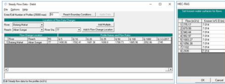
Gambar 36. Inputing kondisi batas steady flow analisist
