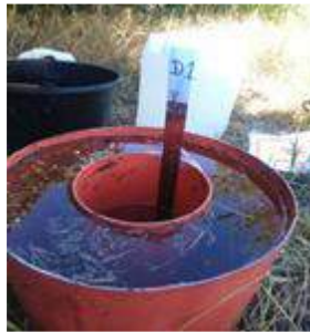
Gambar 4. Double Ring Infiltrometer Laju Infiltrasi
